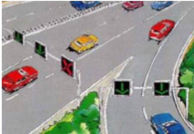
Slika 27. Kontrola spajanja traka u interakciji sa kontrolom priljevnih tokova [Izvor: Texas Transportation Institute Mobility Investment Priorities: Dynamic Merge Control., Strategies Mobility Investment Priorities ]
