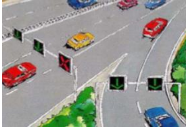
Slika 27. Kontrola spajanja traka u interakciji sa kontrolom priljevnih tokova [Izvor: Texas Transportation Institute Mobility Investment Priorities: Dynamic Merge Control., Strategies Mobility Investment Priorities ]
