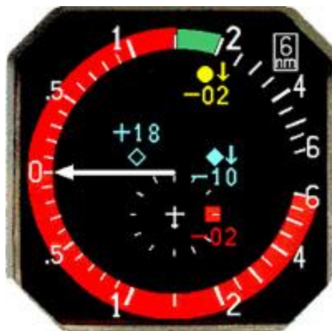
Slika 13. Airborne Collision Avoidance System prikaznik [30]
