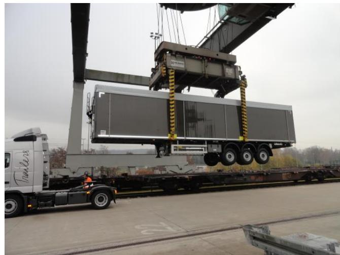
Izvor: Transport of loaded moving floor trailers via rail, Knapen Trailers, <http://www.knapen-trailers.eu/actueel/nieuws/transport-of-loaded-moving-floor-trailers-via-rail>, (pristupljeno 20.07.2016.)
