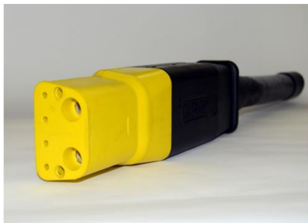
Slika 13: 270V DC zrakoplovni kabel, izvor: http://www.aviationpros.com/product/12237205/mcm-engineering-inc-270v-dc-aircraft-cable
