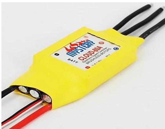
Slika 6. ESC- Electronic Speed Regulator
