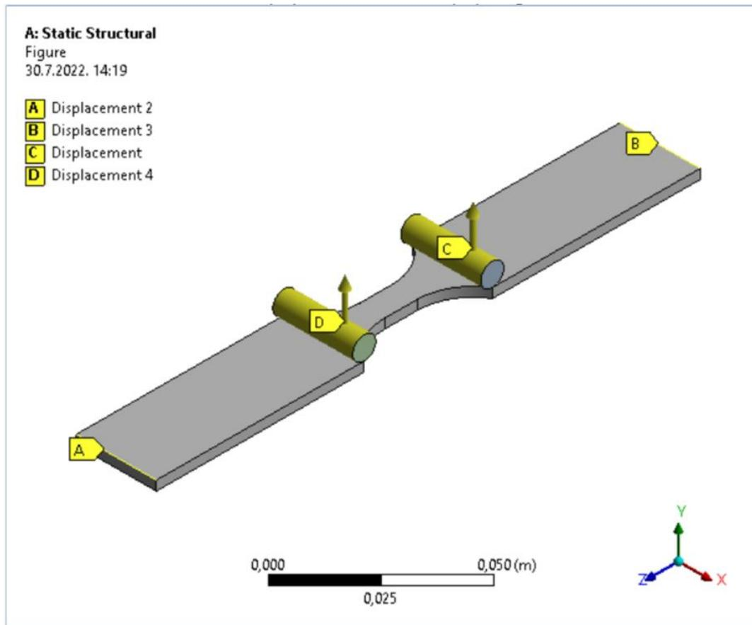
Figure 65. Bending test displacement restriction setup.
