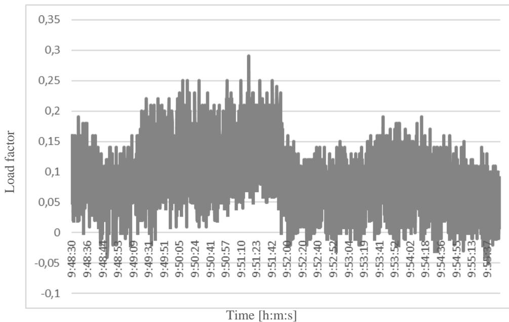
Figure 44. Horizontal flight phase lateral load factor, [4].
