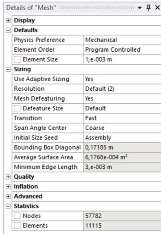
Figure 64. Bending test finite element mesh setup.
