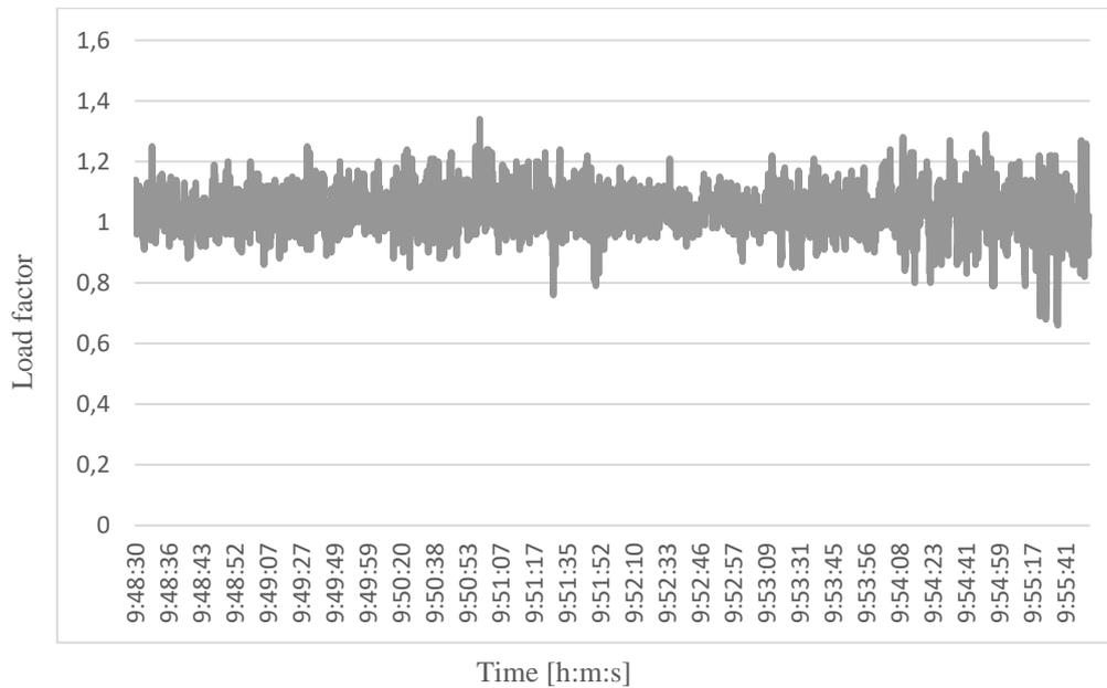
Figure 42. Horizontal flight phase vertical load factor, [4].
