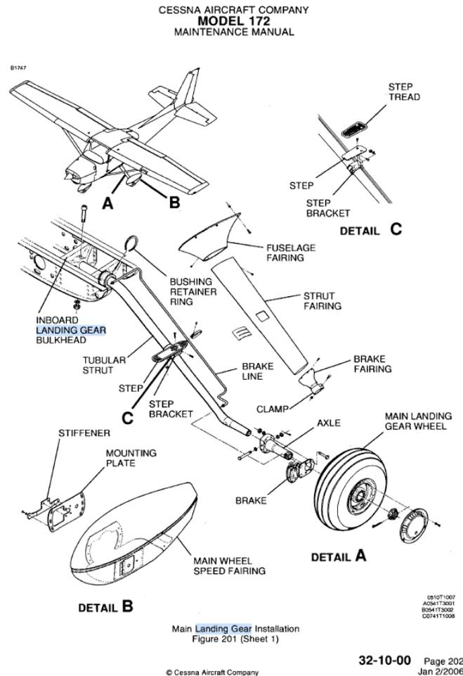
Figure 19. Cessna 172R landing gear assembly, [13].
