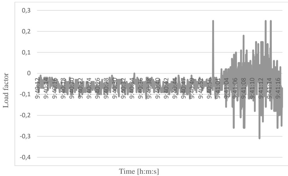
Figure 39. Take-off phase longitudinal load factor #2, [4].
