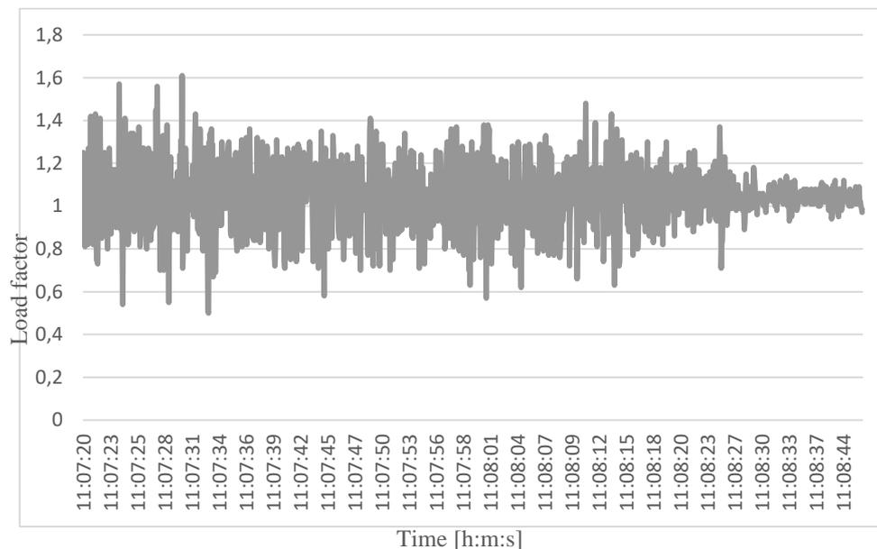
Figure 46. Vertical load factor measurements during airplane landing, [4].
