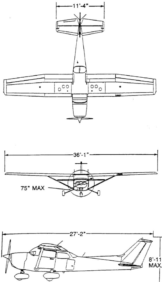
Figure 18. Cessna 172R aircraft three-view drawing, [3].
