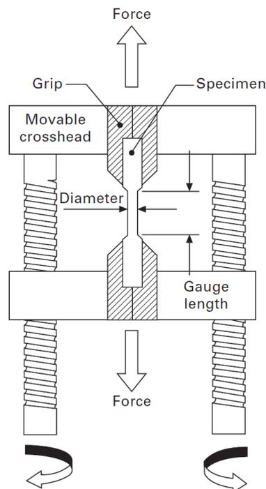
Figure 10. Representation of a tensile loading machine, [109].
