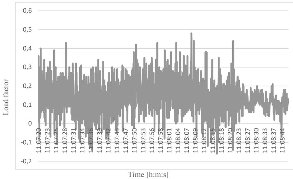
Figure 49. Lateral load factor measurements during airplane landing, [23].
