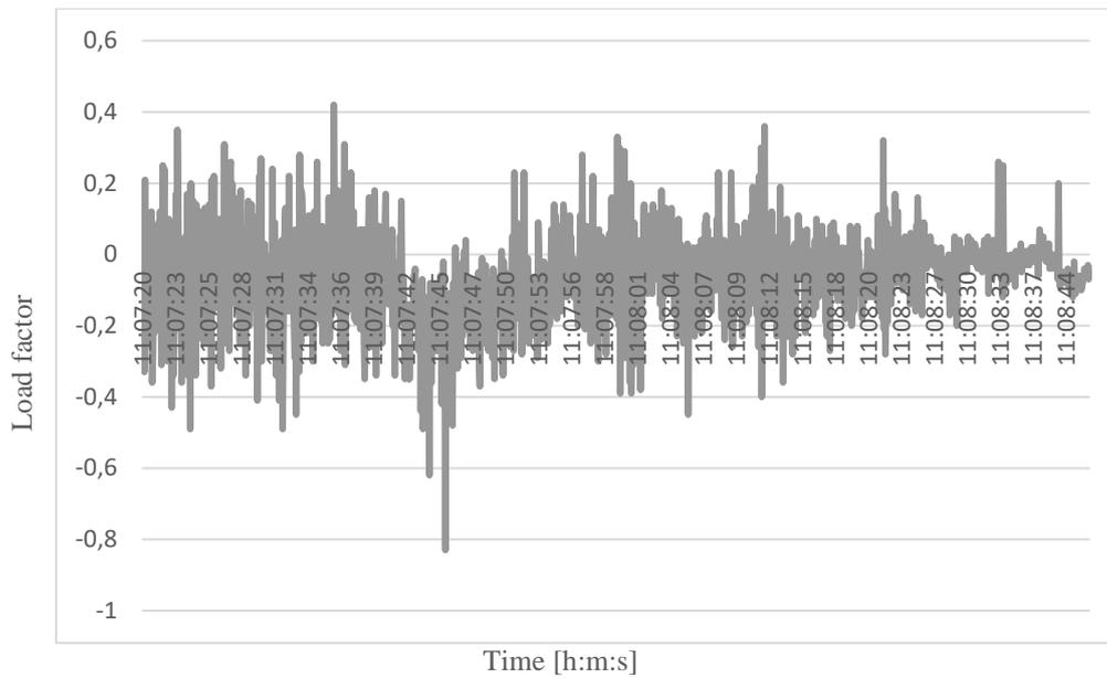
Figure 48. Longitudinal load factor measurements during airplane landing, [4].
