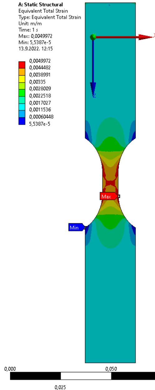
Figure 56. Static structural Equivalent Total Strain [-] tensile simulation results.
