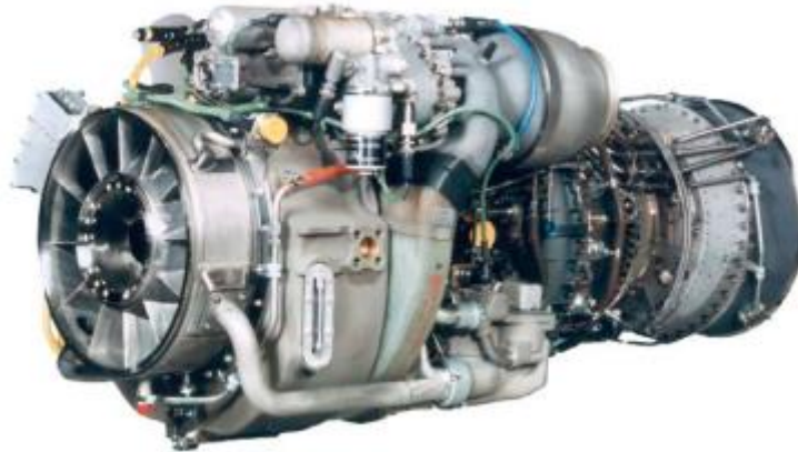
Slika 5: Turbopratilni motor General Electric T700-GE-701D [4]
