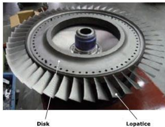
Slika 14. Integrated Blade Rotor, [19]
