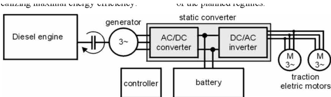
Figure 7: NE train (New Energy Train) series hybrid propulsion
