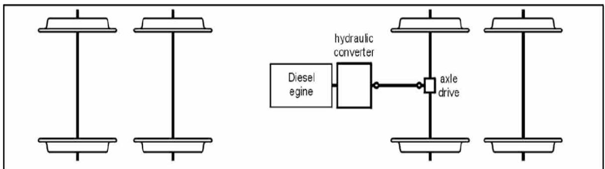
Figure 1: Classical propulsion with hydraulic power transmission
