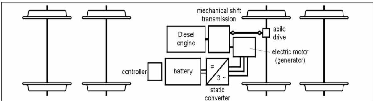
Figure 4. Motor-Assisted (MA) Hybrid Traction System
