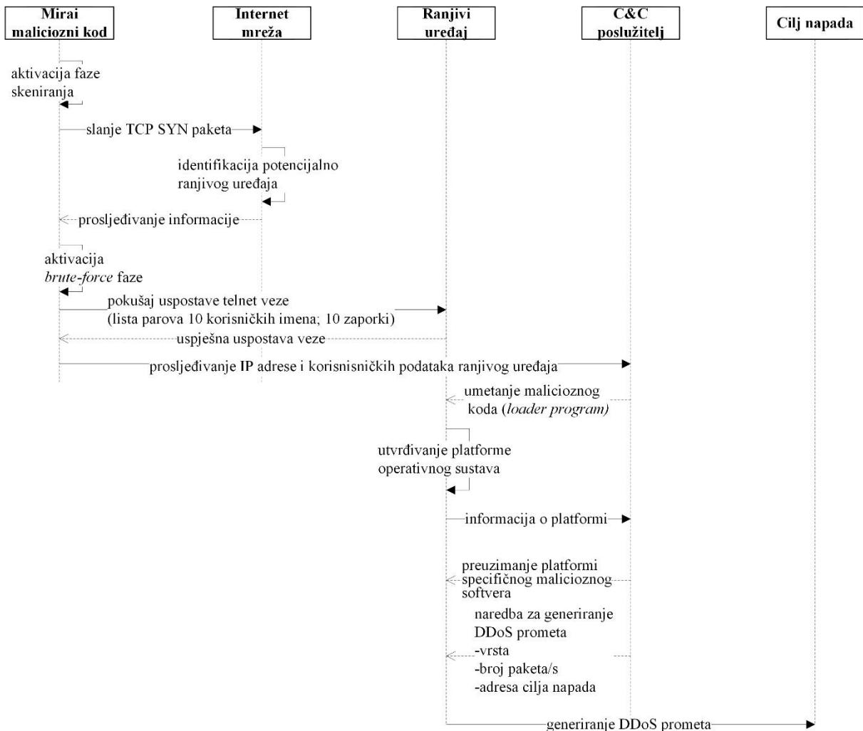
Slika 4.9 UML dijagram principa rada Mirai *botnet-a* [173]
