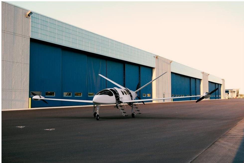
Slika 9. Eviation Alice zrakoplov pogonjen Magni250 motorom [8]
