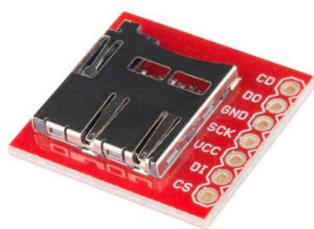
Slika 5.2-5. MicroSD Transflash Breakout pinovi, [33]
