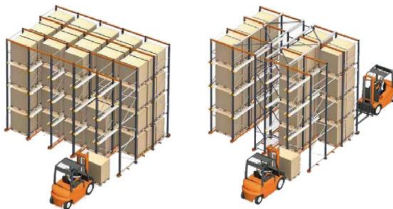
Slika 23: Drive in i drive through regali, [36]
