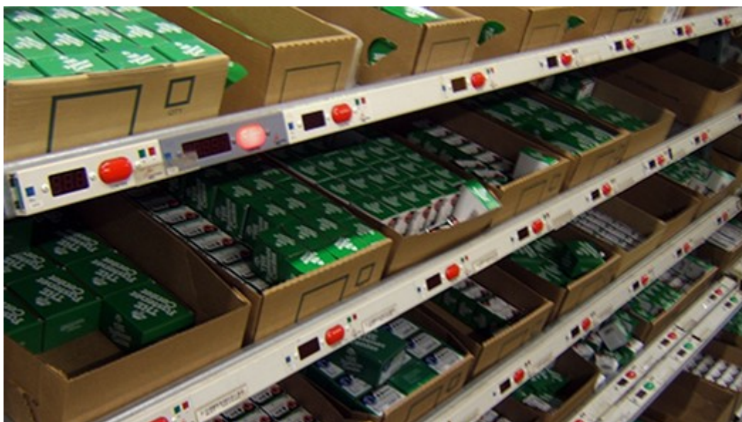
Slika 27. Prikaz Pick by light pull by light tehnologije
