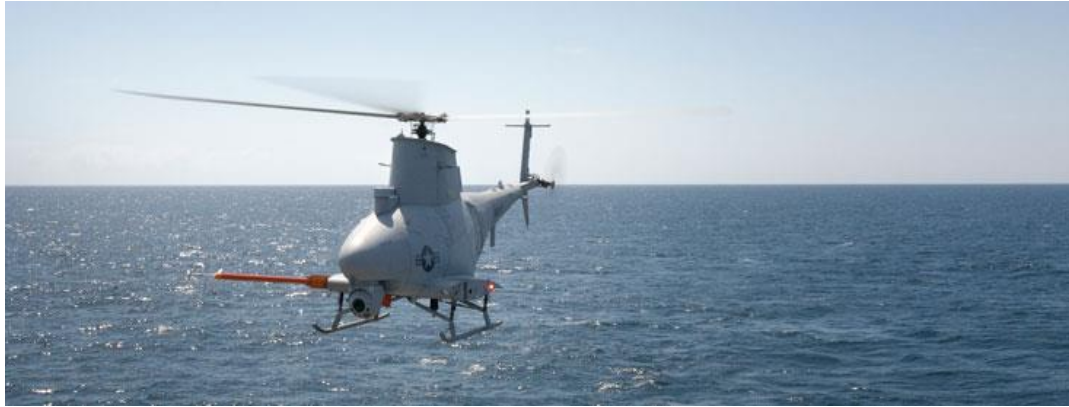
Slika 7. VTOL dron "Fire Scout MQ-8B"
