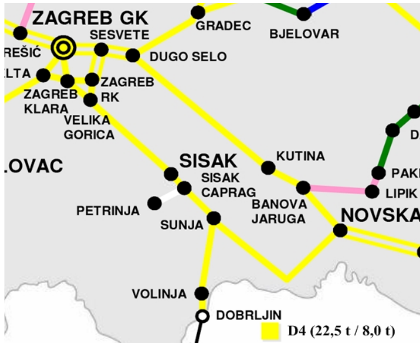
Figure 43. Loads on part of Croatian railway network Source: [8]
