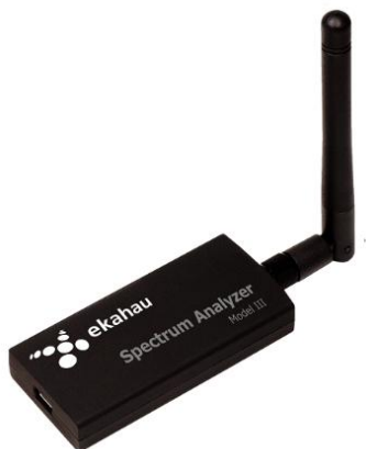
Slika 15. EkaHau dual band USB spectrum analyzer , [25].
