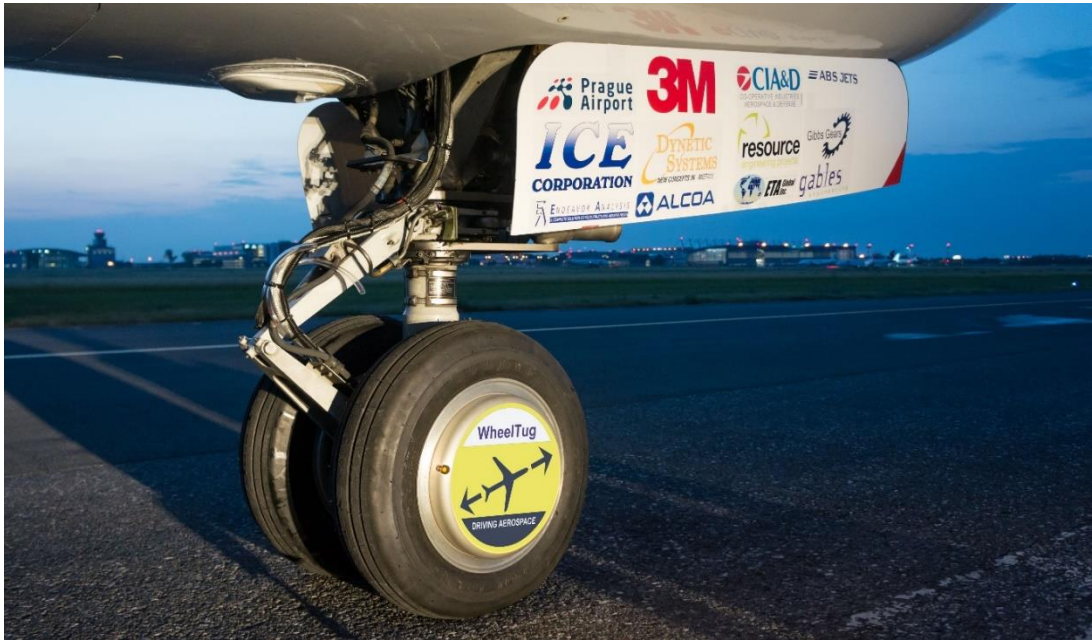
Figure 8. WheelTug system installed on a Boeing 737NG's nose gear 80
