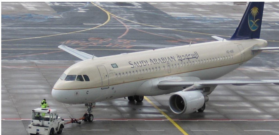
Figure 2. An Airbus A320 aircraft being towed by a classic tug with a tow bar 62
