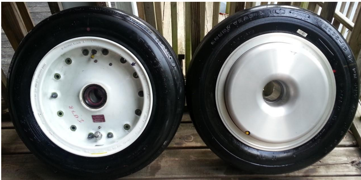
Figure 5. Boeing 737NG nose wheel without (left) and with WheelTug system installed (right) 76
