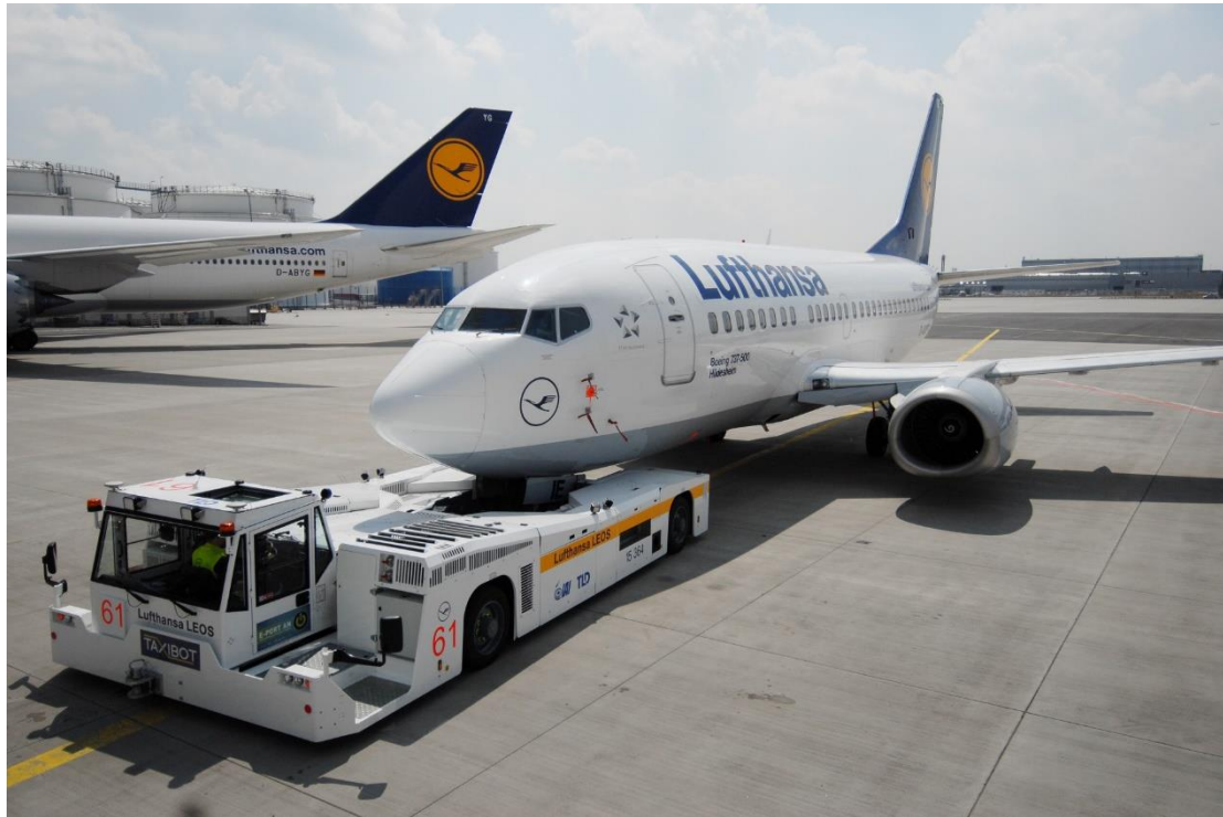
Figure 3. Narrow-body TaxiBot tug 66
