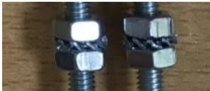
Figure 22- Bolt system to leave a distance between the load cell and the base.
