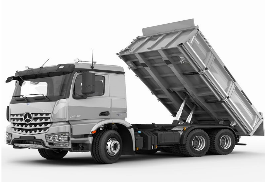
Slika 8. Kamion samoistovarivač marke Mercedes-Benz, model Arocs 6X4 Tipper Izvor: https://www.turbosquid.com/3d-models/arocs-6x4-tipper-3d-model/802573 (travanj, 2018.)
