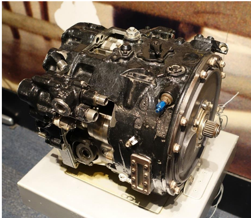
Slika 5: CSD za zrakoplov Boeing 727, izvor: https://en.wikipedia.org/wiki/Constant_speed_drive
