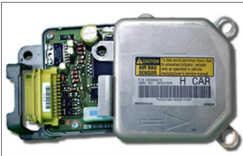
Slika 10. EDR (Event-Data Recorder)
