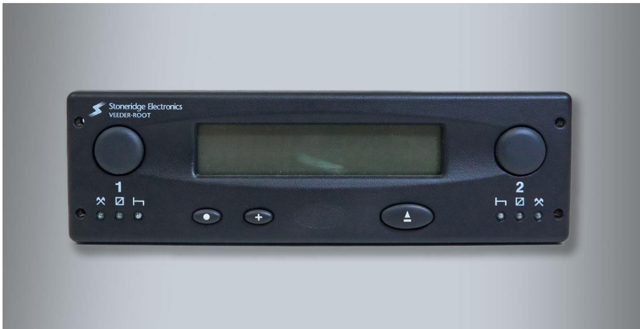
Slika 6. Stoneridge Electronics analogni tahograf, [23]
