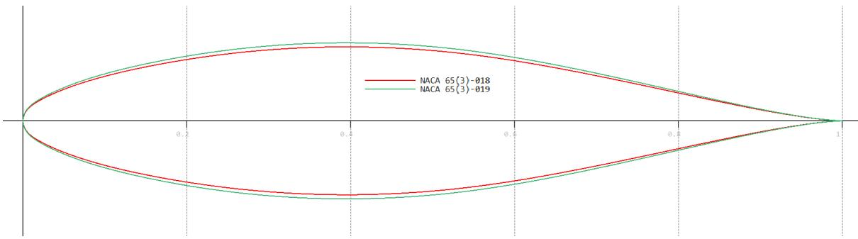
Slika 12 NACA 65<sub>3</sub>-018 i 65<sub>3</sub>-019 u XFLR5.
