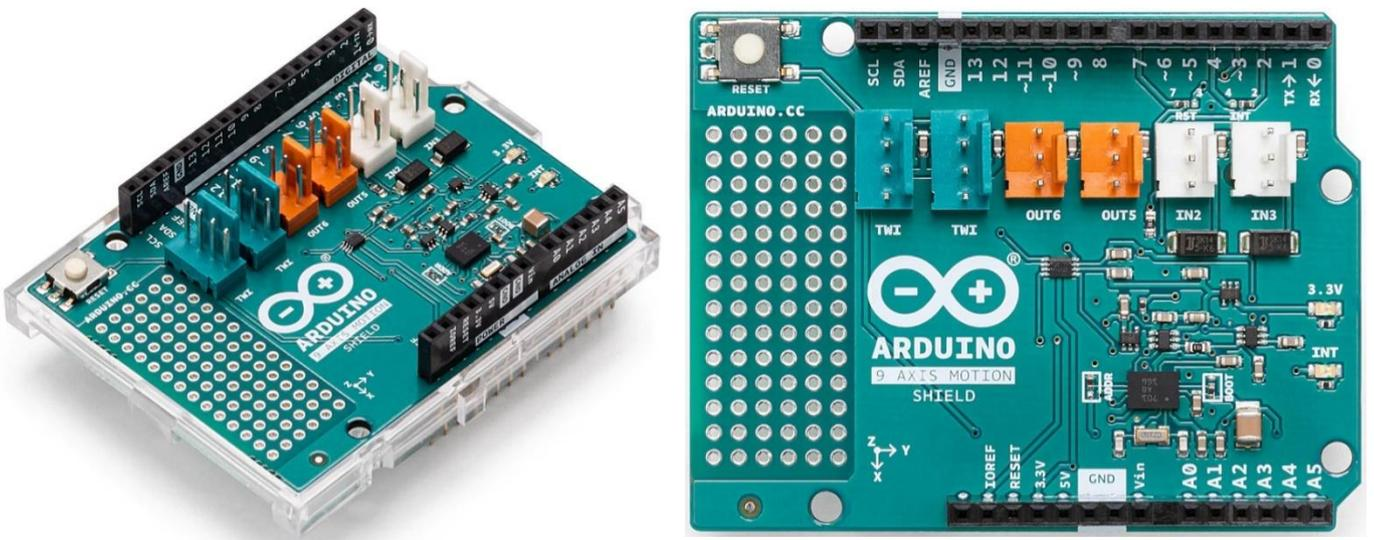
Slika 2. Modul 9 Axis Motion Shield. Izvor [24]
