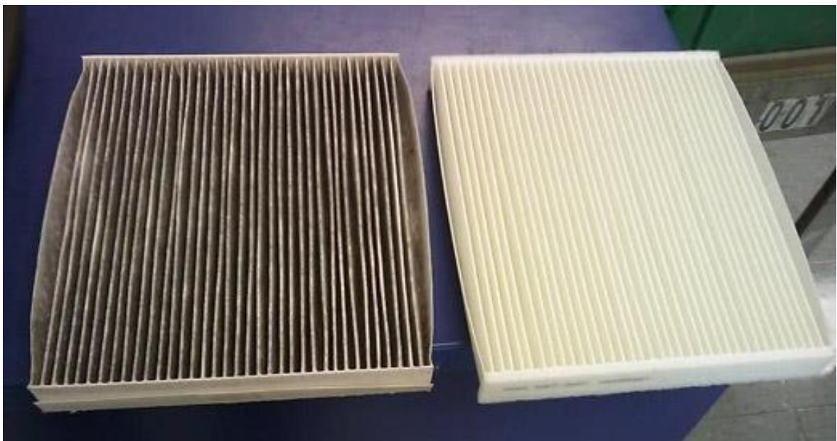
**Slika 16.** Dotrajali filter kabine i novi filter kabine
