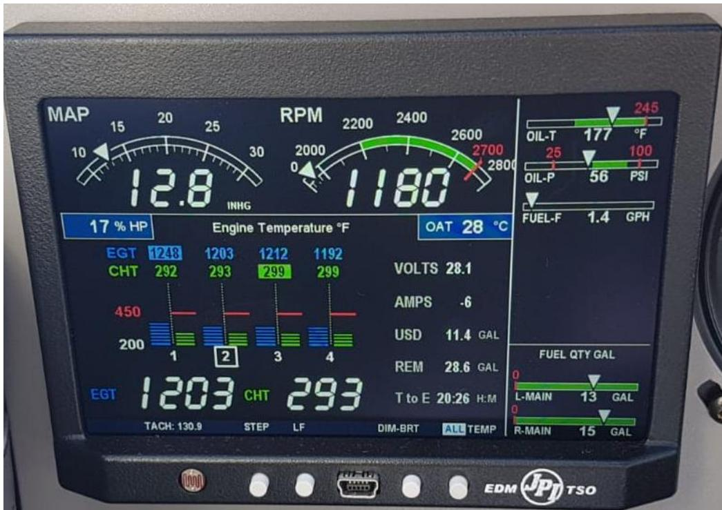
**Slika 8.** Motorski instrument EDM-900
