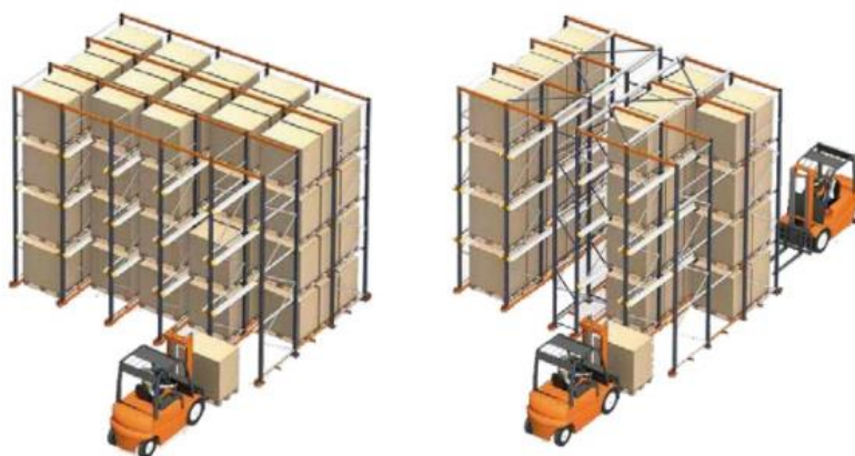
Slika 23: Drive in i drive through regali, [36]
