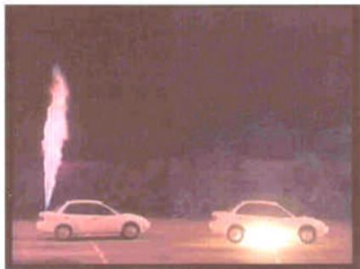
Photo 2 - Time 0 min, 3 seconds - Ignition of both fuels occur. Hydrogen flow rate 2100 SCFM. Gasoline flow rate 680 cc/min.
