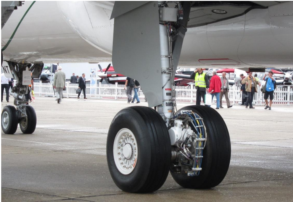
Figure 4. EGTS system mounted on an Airbus A320's main landing gear 69
