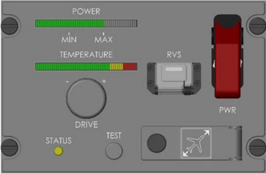
Figure 7. Publicly available WheelTug cockpit panel design 79
