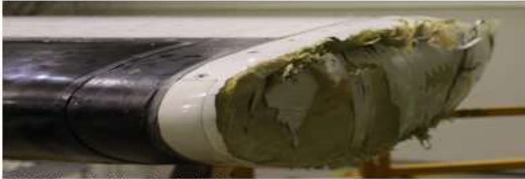
The left horizontal stabilizer tip at the aircraft
