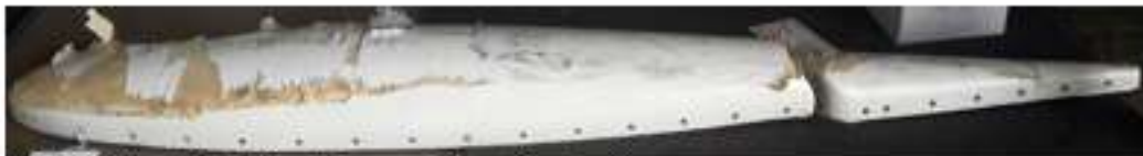
The left horizontal stabilizer tip removed from the aircraft
