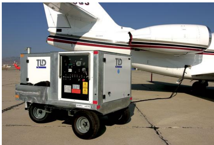
Slika 2: GPU (Ground Power Unit)
