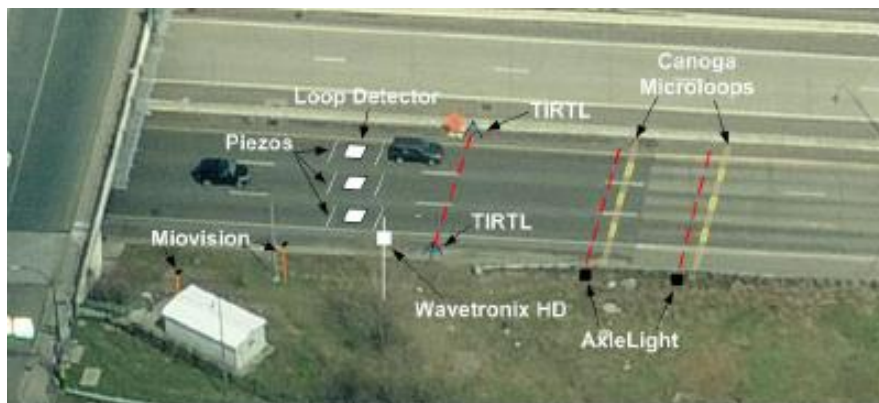
Figure 2 Traffic detectors (source: Ohio state university, April 2016)
