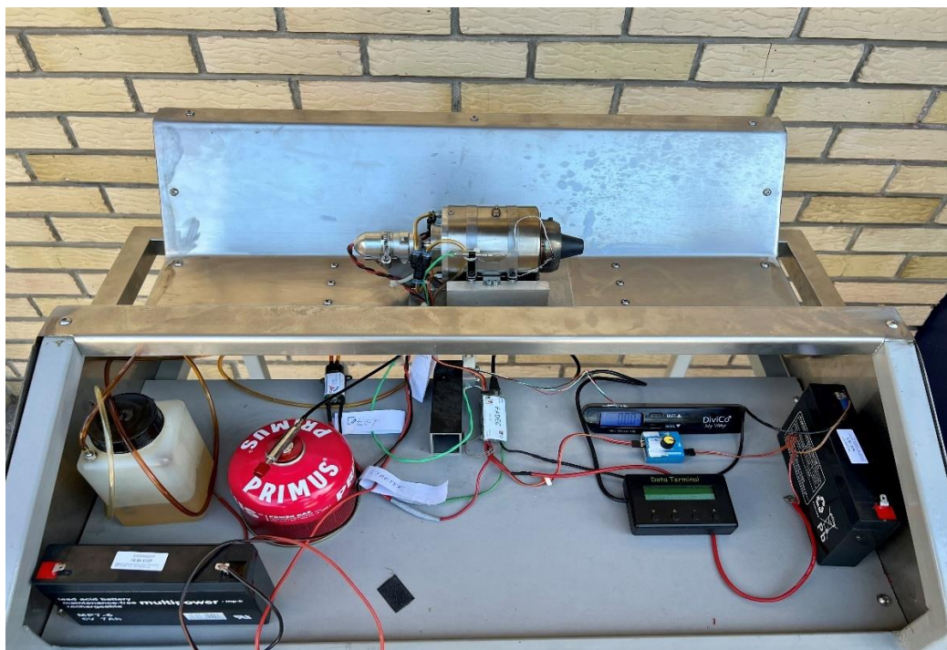
Figure 13 Test bench with the JJ1400 engine, sensors, and data terminals
