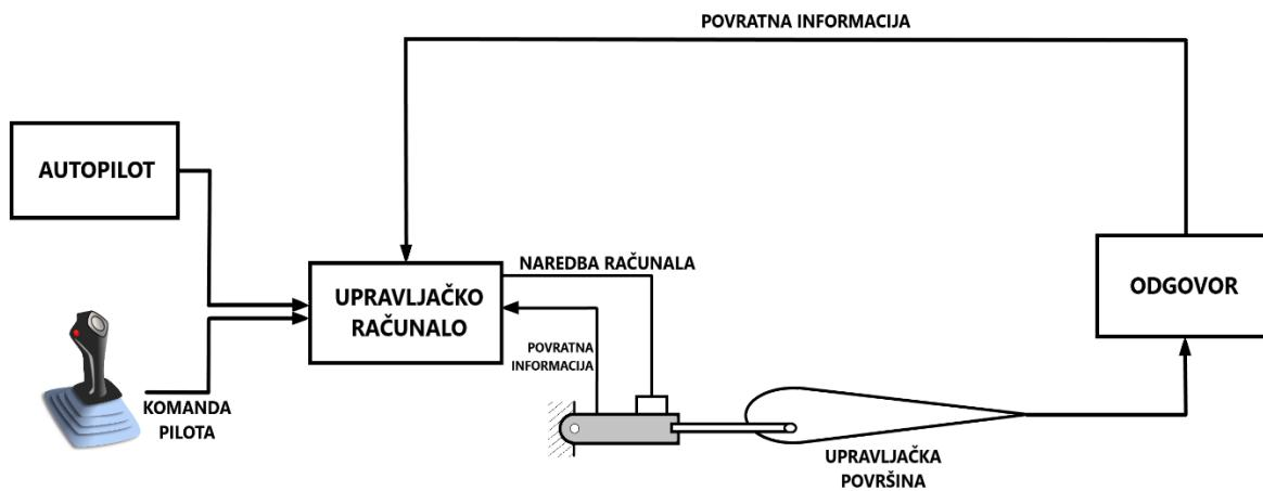
**Slika 11.** Shema sustava Fly by wire
