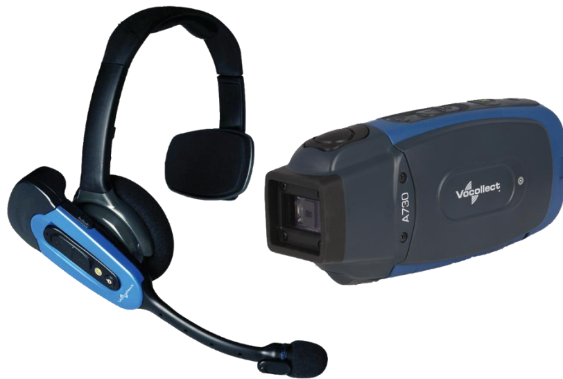
Slika 22. Prikaz Pick by Voice opreme
