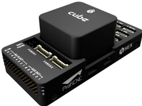
Slika 13 Pixhawk autopilotski modul, model 2.1 [21]
