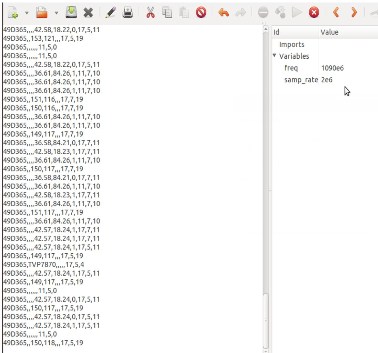
Slika 18: Dekodirane ADS-B poruke
