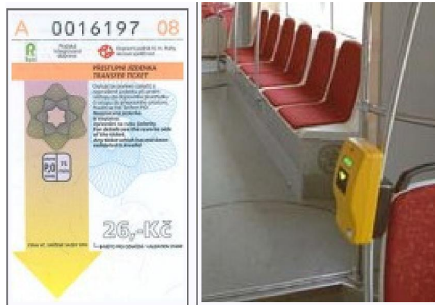
Slika 1. Papirnata karta i uređaj za validaciju Izvor: Ticketing for public transport ( Stadium - ITS for large events)
