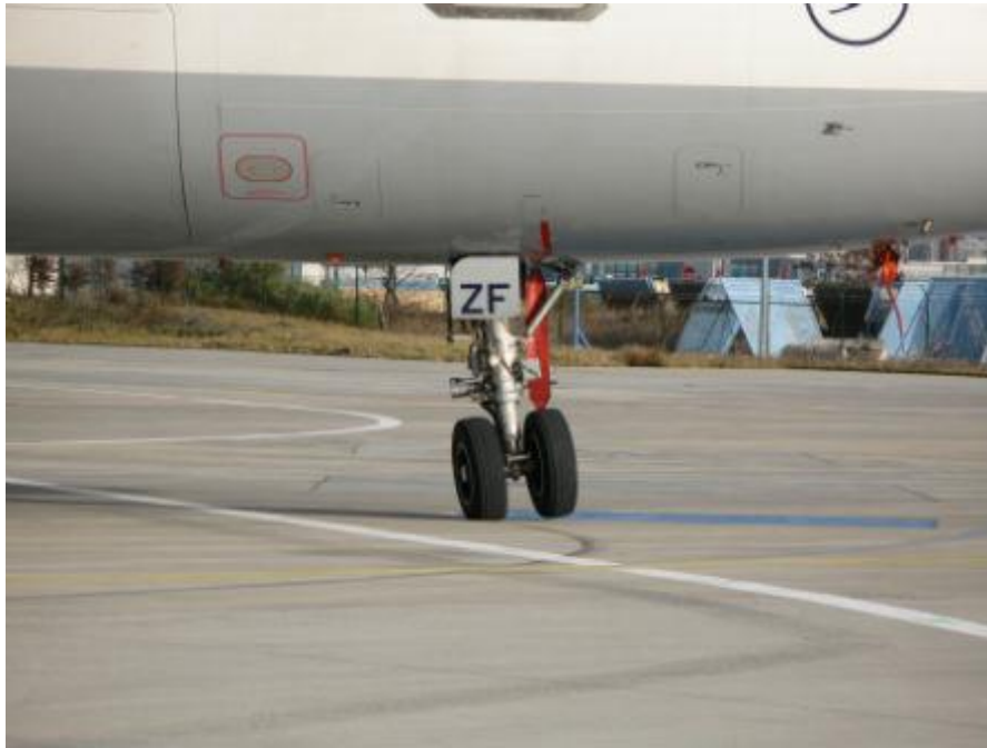
Figure 9. Airbus A320 nose wheel lifted of the ground during a tight turn 81
