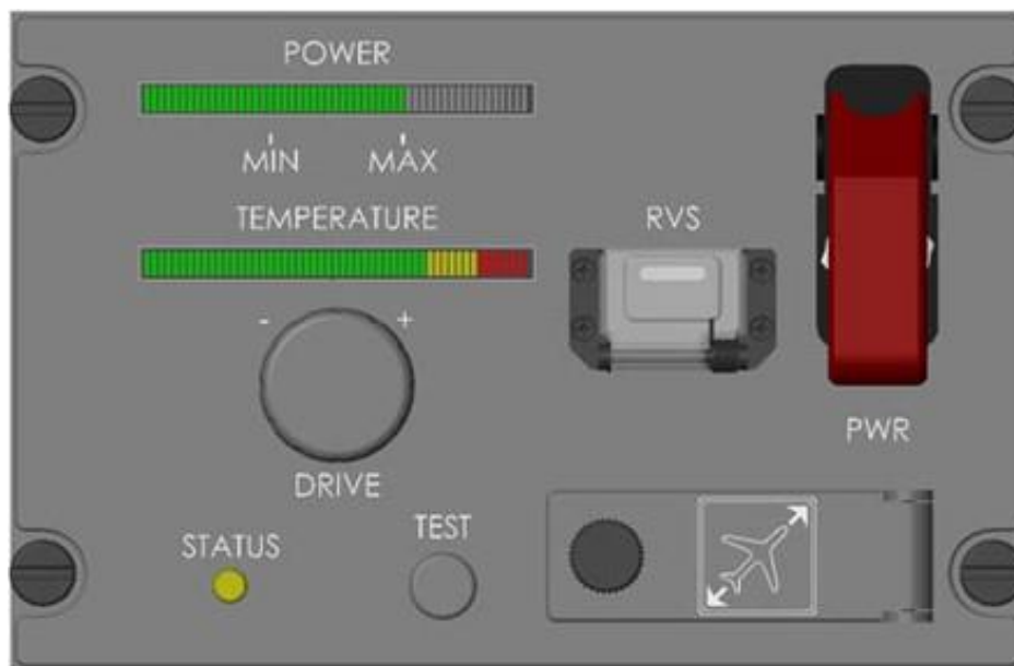
Figure 7. Publicly available WheelTug cockpit panel design 79
